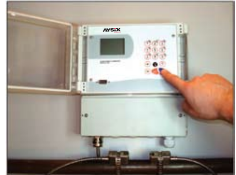
Aysix 150 wall-mounted with transducers
